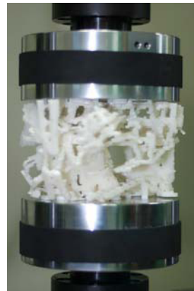
Fig. 5. Experimental compression test with INSTRON test machine.
